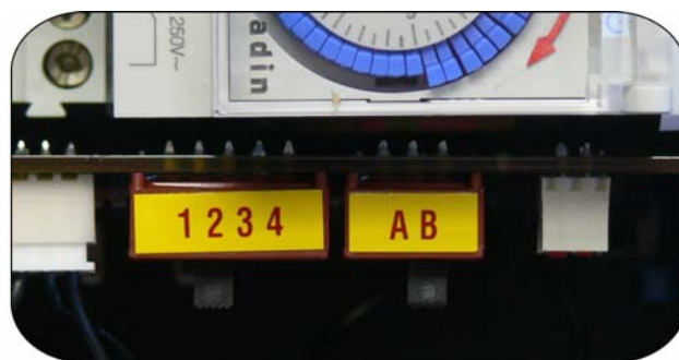
Figure 3. '1' = Frequency 1 (2–4 min.); '2' = Frequency 2 (4–8 min.) '3' = Frequency 3 (8–16 min.) '4' = Frequency 4 (16–32 min.) 'A' is quiet volume sound setting; 'B' is loud volume setting.
