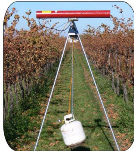
Figure 1. This side view of a bird banger shows the cylindrical barrel at top, open on one end (right side in photo), control system box (top, back), tripod and tank of propane gas.
